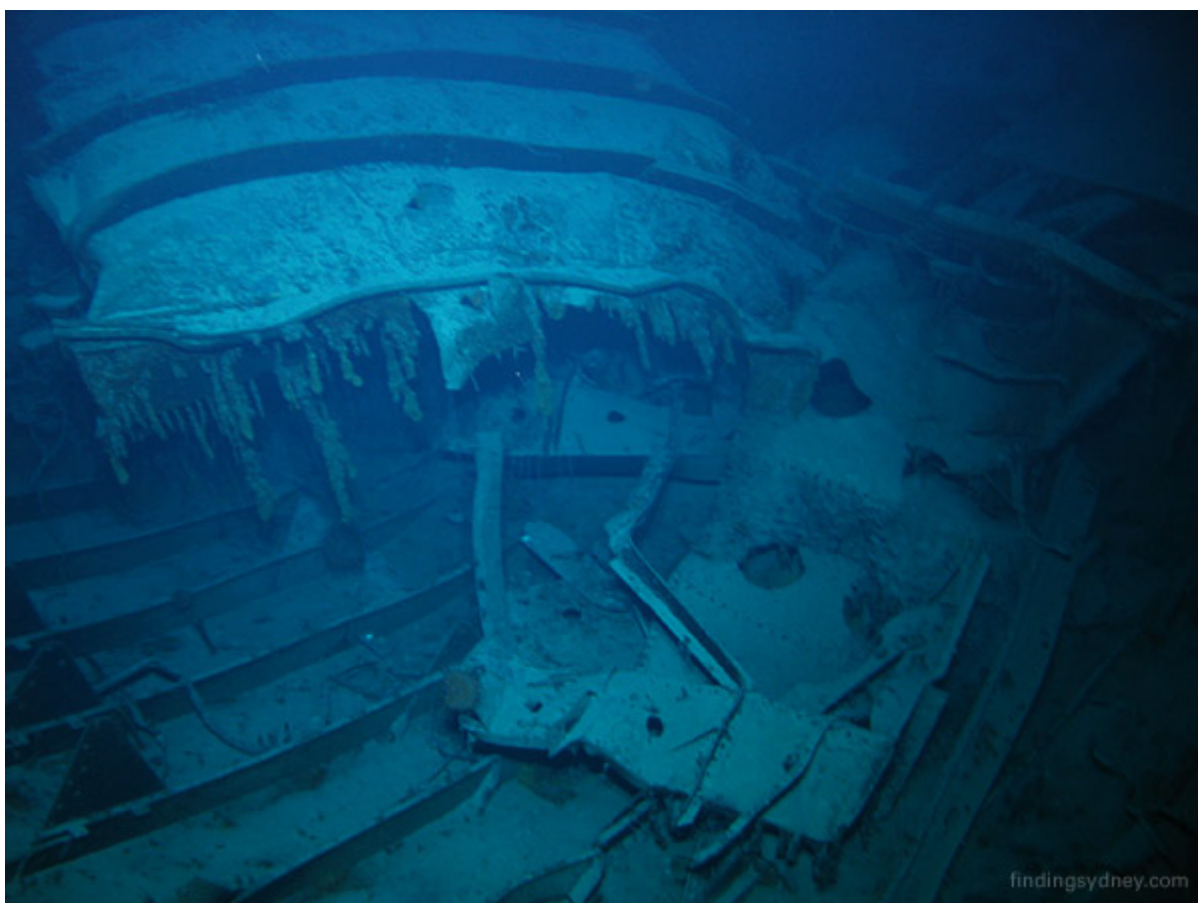
Above Photograph: 5.9 Gun: Kormoran's 5.9-inch gun in the forward hold pointing to starboard and aft of the beam.
