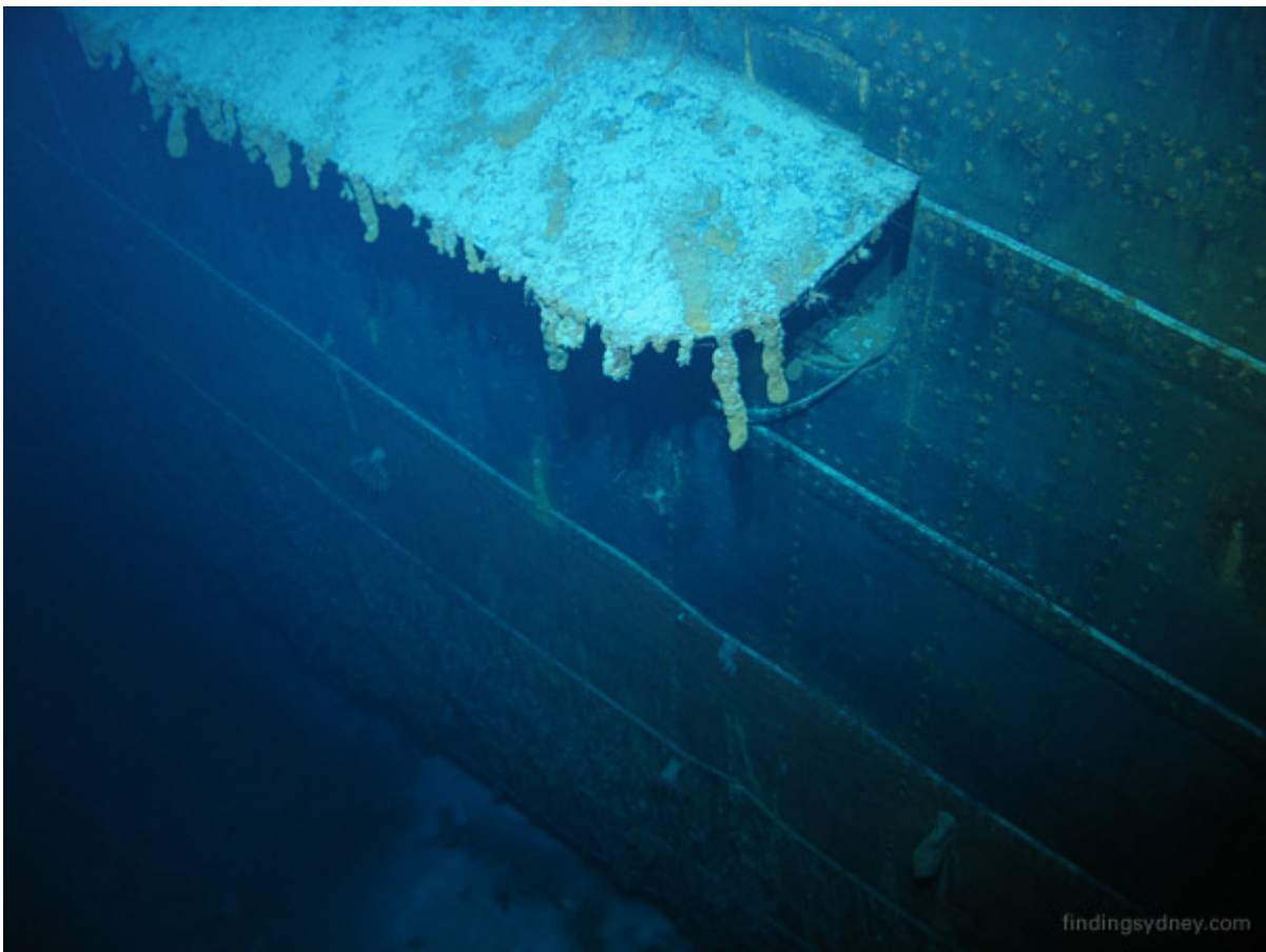
Above Photograph: The simple flap designed to conceal the starboard and port above-water torpedoes shown here on the starboard side in the open position.
